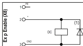
This circuit variant is used for DC-powered relays / contactors. A diode is connected in the reverse direction parallel to the coil.
