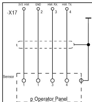
The optionally available p operator panel may be connected to terminal row "X17".
