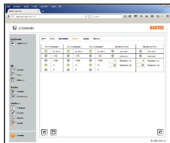
The temperature sensors are configured in the “Extended / Sensors” menu.
