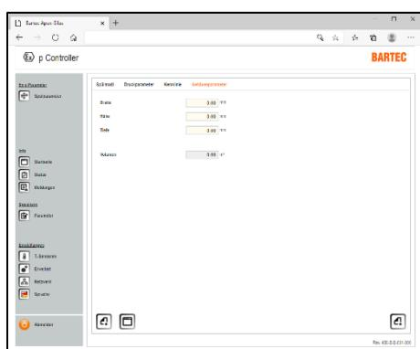
The internal volume of the pressurised equipment is specified in the “Enclosure parameters” tab.
