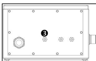
A 10 mm pipe connection is available for activating the mpv (3)
