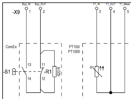
So that the bypass switch is recognised, and the function can be carried out, a resistor with 620R must be connected to the closing contact.
