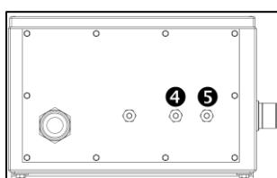
The pressure measurement connections "I internal pressure" (4) and "L mpv pressure" (5) are each designed with a 10 mm pipe connection.
