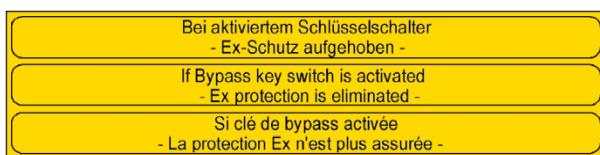
The position of the bypass key switch is queried by the control electronics in an intrinsically safe manner.
