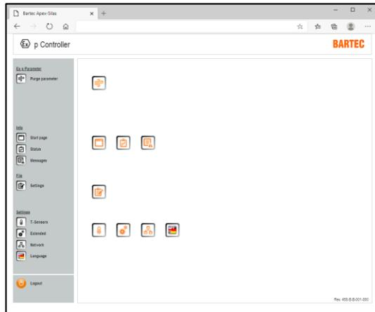
You can jump directly to the specific submenus by clicking on the grey navigation bar on the left.
