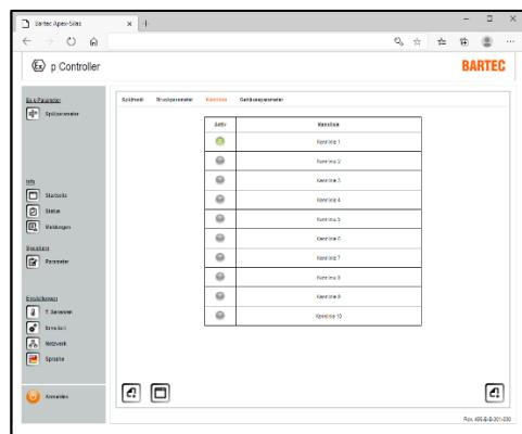
The application-specific mounted pressure monitor is specified in the “Characteristic curve” tab.
