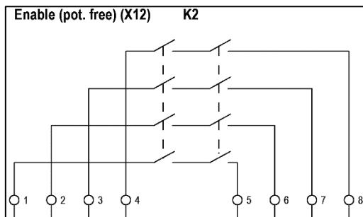
A potential-free message (4x NO) is available on the APEX / SILAS control unit. This message can either be used as a release, which is also safety-related. Or used as a potential-free message. Switching values for the relay can be assigned individually.
