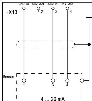
Pressure or gas sensors with a 4... 20 mA output may be connected to sensor input OS 2 [Ex ia].
