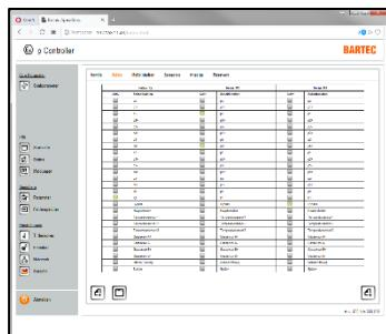
In the “Extended / Relays” menu, the switching points can be assigned to the relays K2, K3 and K4.
