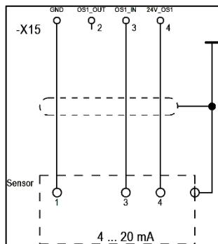
Pressure or gas sensors with a 4... 20 mA output may be connected to sensor input OS 1 [Ex ib].
