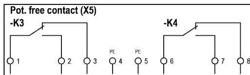
A potential-free changeover contact K3 and K4 is available on the Ex p control unit for reporting and processing signals. The associated switching function can be set in the Ex p control unit via the WEB interface and is freely programmable. The maximum switching current is 1 A.
