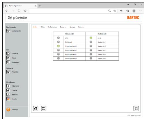
The inlet and outlet valves are preset on the Ex p control unit APEX<sup>mpc</sup> or respectively on the SILAS<sup>mpc</sup>. The settings should not be changed, otherwise the function is no longer guaranteed.
