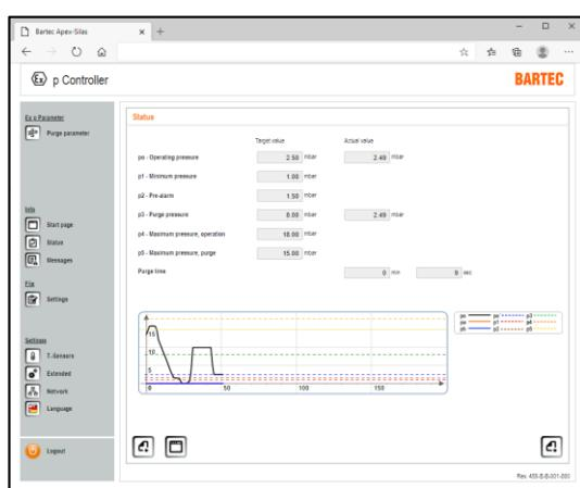
In the lower area of the submenus, there are three icons which fulfil the functions Forward / Back and Home.
