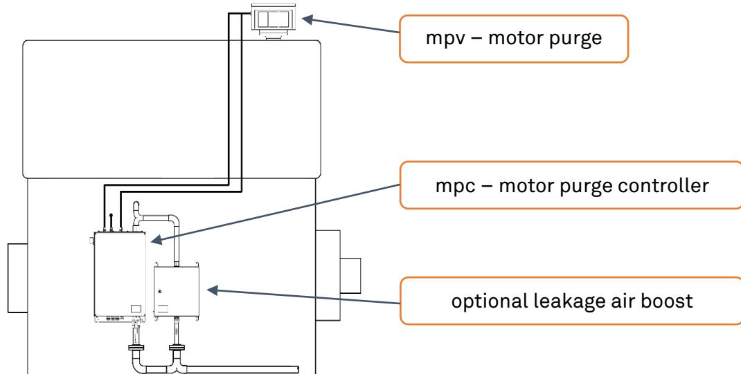
The APEX<sup>mpc</sup> or SILAS<sup>mpc</sup> is attached to the motor with the additional system components, e.g. leakage boost, on the outside of the motor using the fastening straps located on the housing.
