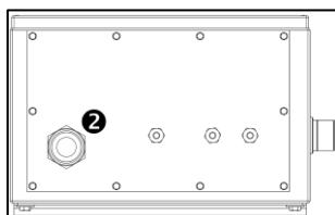
The purge gas supply (2) from the motor purge controller to the protected motor is designed with a G 1 ½ "external thread.
