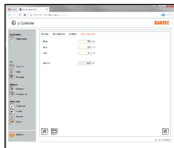
The internal volume of the pressurised equipment is specified in the “Enclosure-related parameters” tab. For this purpose, length, width and height must be entered in mm.
