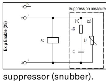
This circuit variant is used for inductive loads and AC-powered relays / contactors. In this circuit variant, the property of the VDR resistor is used to become low-resistance above a certain threshold voltage. This short-circuits the self-induced voltage. The resulting vibrations are damped by the RC suppressor (snubber).
