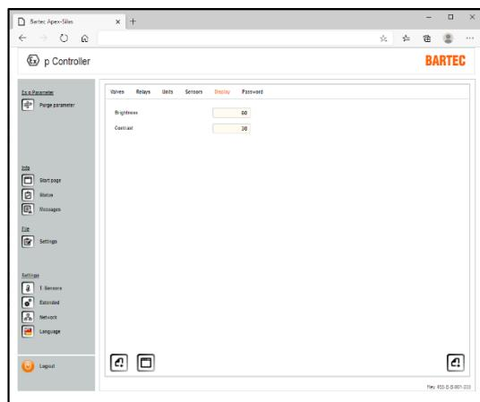
The contrast and brightness of the LCD display on the p-Operator panel can be set in the “Display” tab.
