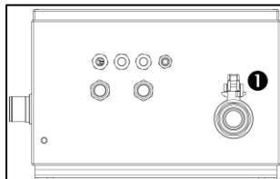
The purge gas supply (1) on the motor purge controller is designed with a G 1 ½ "internal thread connection.
