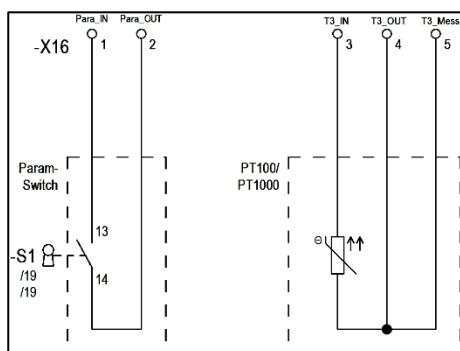
The BARTEC parameter switch must be used to change parameters.
