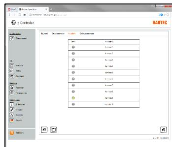
The specifically mounted pressure monitor is specified in the “Characteristic curve” tab. This must be set correctly for the correct automatic purge time calculation.
