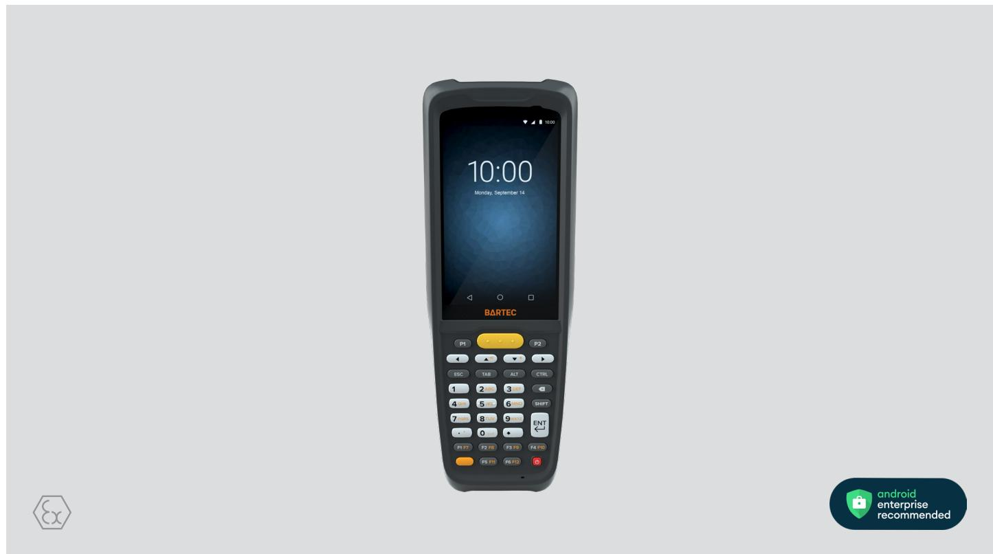
BARTEC has developed in close cooperation with Zebra Technologies the MC27<sup>ex</sup>-NI for worldwide use in hazardous areas.
