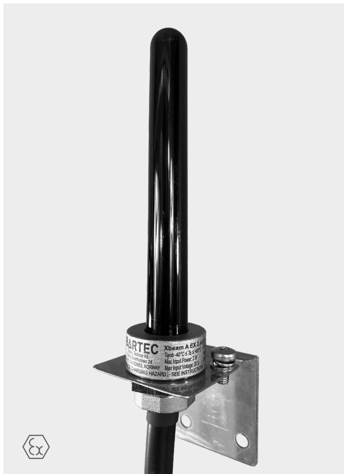
The Xbeam™ A EX is an ATEX and IECEEx approved RF antenna for creating wireless networks (typically Wi-Fi and Bluetooth) and wireless telemetry systems in hazardous area. The antenna is not limited to a specific network protocol and can be used for any 2.4GHz and 5.0GHz application. The antenna is optimized for use in steel and concrete structure environments where multipath effects and reflections are present.
